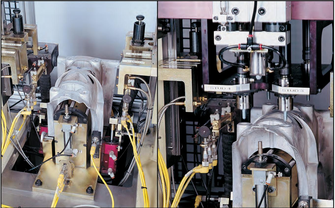
**Fig. 2** – A magnesium shift tower for a new line of SUVs from General Motors is shown at an assembly station where Mag-Form fasteners compress threads into four cored holes.
