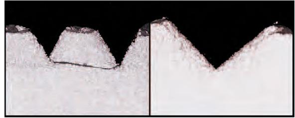
**Fig. 4** – The 60-degree flank angle on the standard fastener exceeds the ductility limit of the material, damaging formed threads and creating debris. (L) Mag-Form fasteners compress rather than roll form threads, eliminating thread fractures and debris accumulation. (R)
