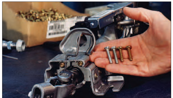
Fig. 1 – Textron Fastening Systems Mag-Form Thread Forming Fasteners (right) replaced the longer Tap-tite roll forming fasteners (left) at the DaimlerChrysler Toledo Machining Plant.
